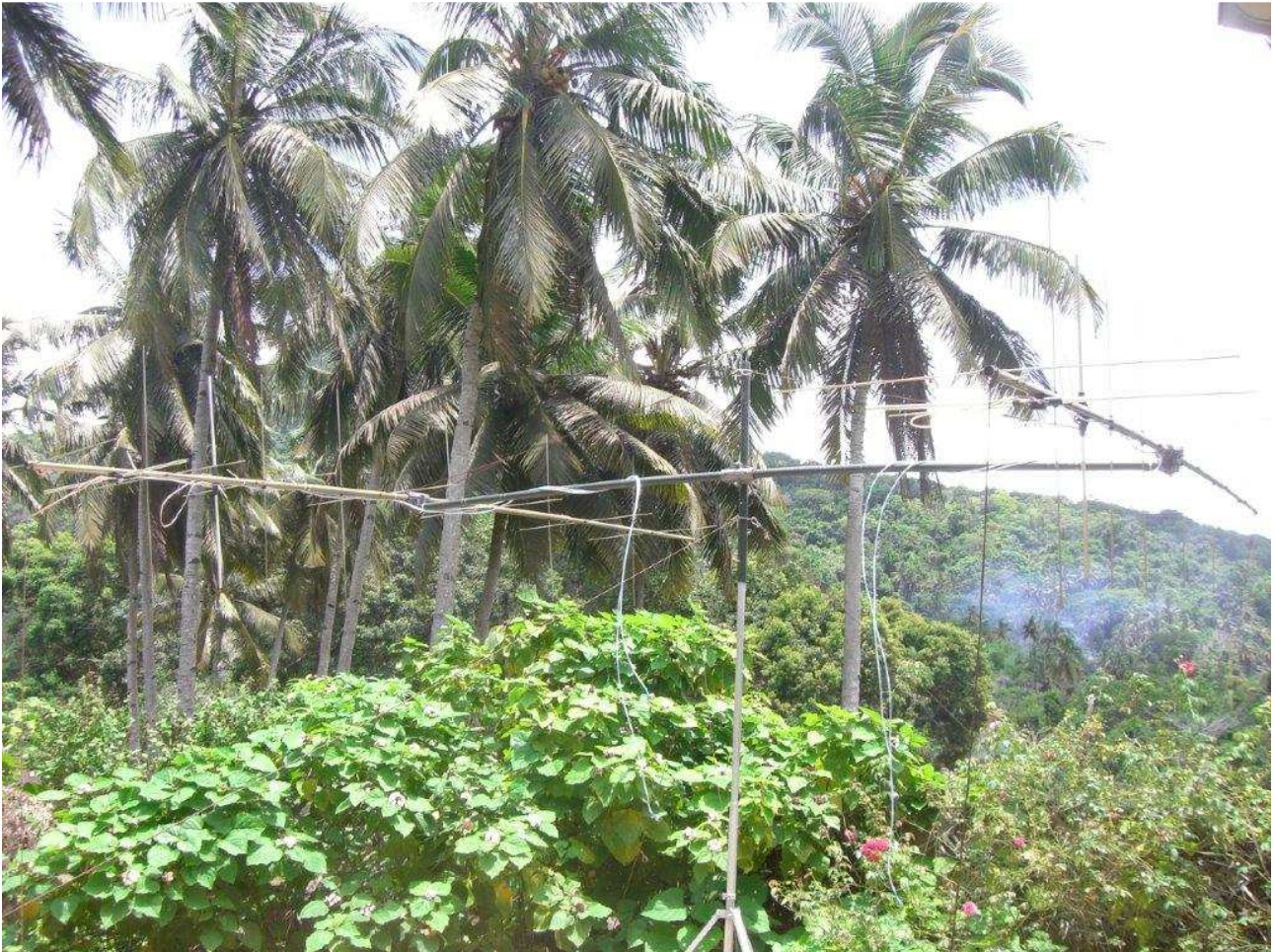
Antennas in the jungle; the hill in the background was the reason for the minimum elevation at moon-set.
