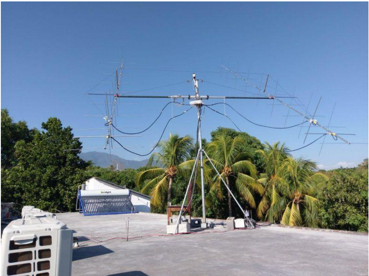
The 2 x 10/10 ele homemade xpol yagis (DK7ZB design) on the hotel roof.
