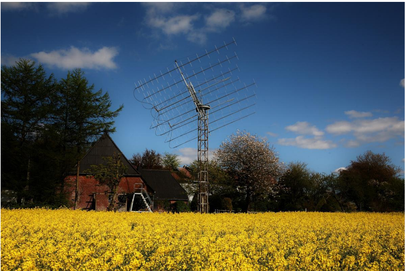
Beautiful antenna in beautiful North-German scenery: the eight 32 ele xpols of DK5LA (Photo DK5LA)
