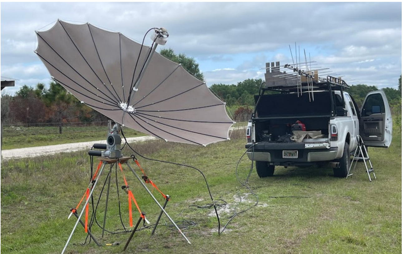
KA6U's 23 cm antenna. Note the 2 m yagis on top his car waiting to be brought into good use again.
