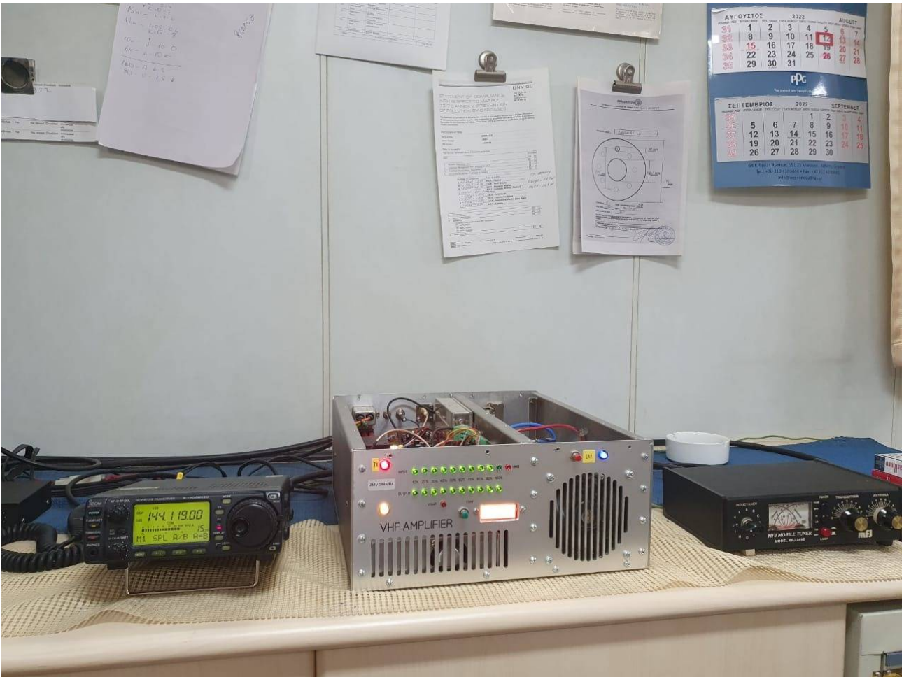
UT1FG/MM's shack onboard the Barnacle: IC706MKII, homemade sspa ~250 W out.
