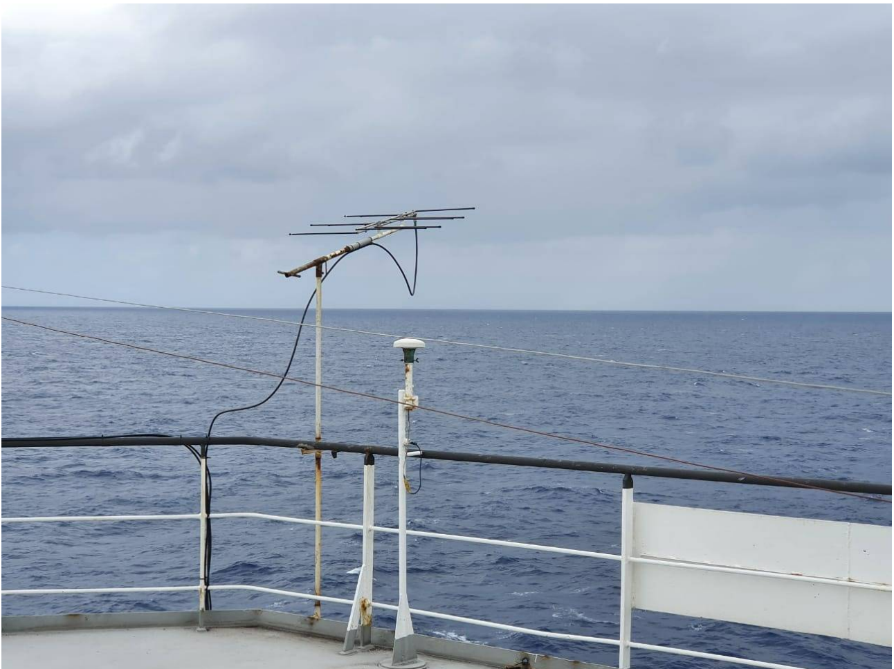
UT1FG/MM's very short antenna onboard the vessel Barnacle. Elevation is fixed at \sim 15^\circ
