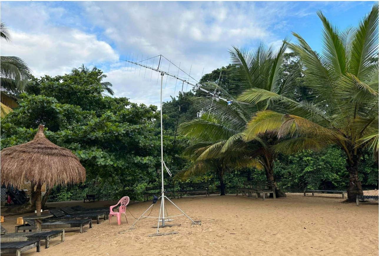
TJ9MD's 2 x 15 ele xpol by Antennas Amplifiers (Photo DL8JJ)
