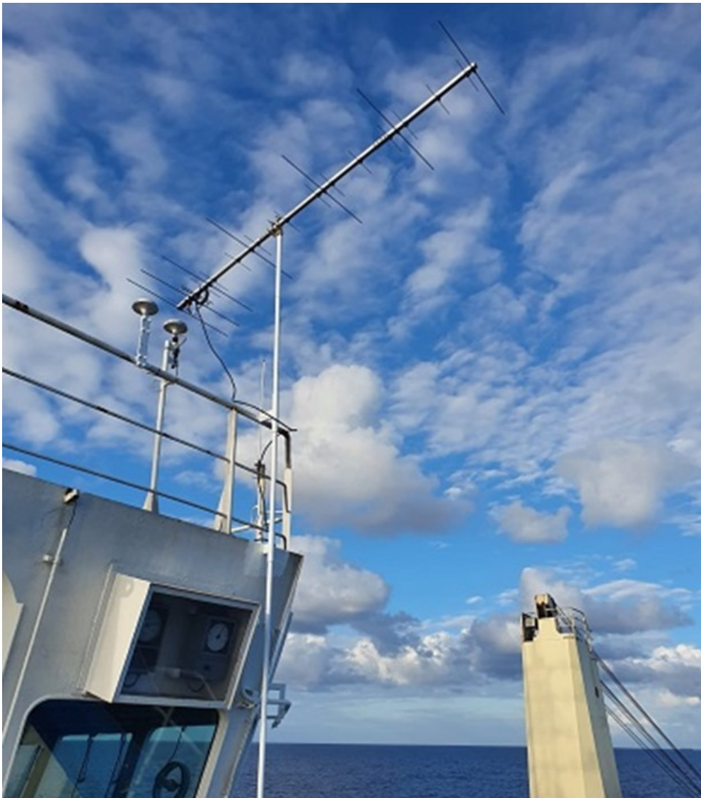
The 7/14ele yagi on board the BRANT.
